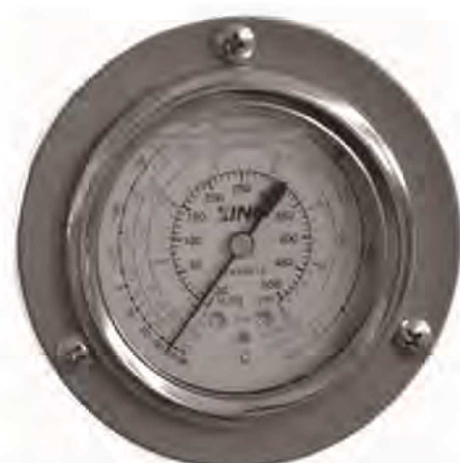
Freon-high pressure gauge
